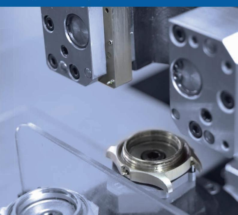
MAGIC is a bench-type machine with 3 axis dedicated to watchmaking for drilling spring bar holes. **This machining concept is unique in the world**. The MAGIC process is to drill simultaneously two spring bar holes perpendiculary between lugs.
